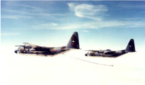
▲ RAF C130s in formation with refuelling hose trailing. Photo courtesy of the Marshall Group
